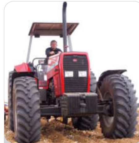
Centre-drive 4-wheel drive front axle gives excellent manoeuvrability
