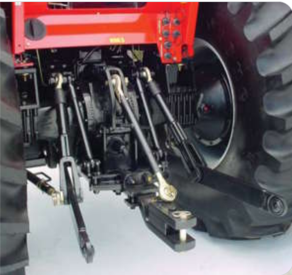
MF 660 rear linkage. The massive rear axle is also clearly shown
