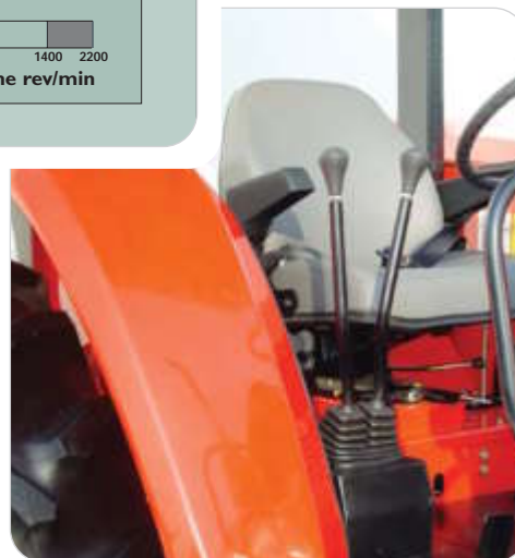
Rubber-mounted platform with side-shift gear levers
